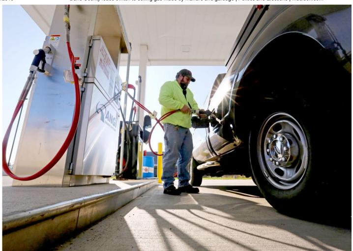
Dane County landfill manager Paul Howard fills his vehicle with compressed natural gas. The gas is collected from the landfill and compressed for use in specially-outfitted vehicles. The county plans to begin selling the gas through an interstate pipeline. JOHN HART, WISCONSIN STATE JOURNAL
